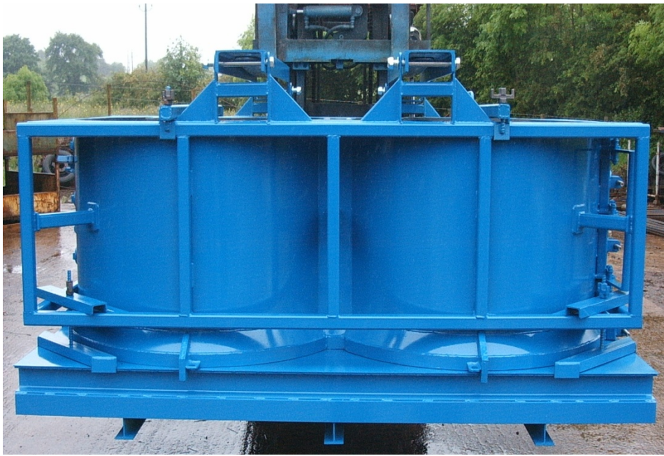
ABOVE: SEPTIC TANK MOULD
