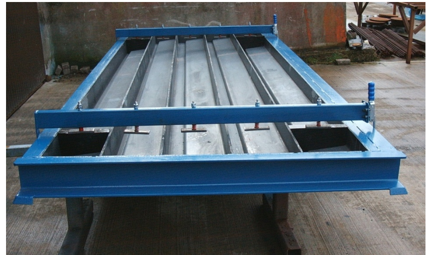
WINDOW CILL MOULD
